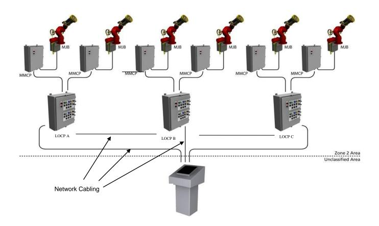
Mesh network: This is the most complete and reliable network configuration and is shown above. Each panel is connected to every other panel. This provides the greatest reliability as multiple links could be lost and the network will still operate by communicating through another path. Note that as supplied there are only two fiber ports installed in the HMI. If additional ports are required for implementing radial or mesh networks a spare managed switch or special order will be required.
