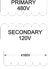
A simple single phase transformer would have two wires going in (primary wires) and two wires coming out (secondary wires). This example is a 480/120 step-down transformer. The term step-down means it lowers the voltage as opposed to a step-up transformer that would be used to raise voltage.
