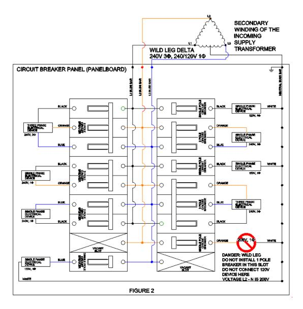
If this were a regular 3 wire 240V delta, or a corner grounded delta, the phase connections (L1, L2, & L3) would be as shown in figure 2. Neither of those transformer styles would not have a neutral conductor. The neutral buss would probably still exist in the circuit breaker panel, but it would be unused. Three phase, and single phase line to line voltages would still be available. Line to neutral would not exist, because there is no neutral. Single pole breakers would not be used.
