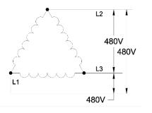
The simplest three phase power system is achieved using the 3 wire delta, which as its name implies has three phase conductors. Three phase power is available by connecting to all three of the phase conductors, L1, L2, & L3. In this example, that would provide 480V 3  $\Phi$  ( $\Phi$  symbolizes number of phases).
