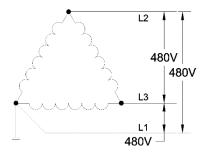
A variation on the normal delta system is the corner grounded delta, where one phase is intentionally tied to ground. While far less common than the one above, it is still relatively popular. The grounded phase conductor should be color coded white, or natural grey. In the U.S. the grounded leg is marked white to indicate that it is grounded, not to indicate that it is neutral.
