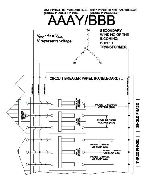
WYE TRANSFORMERS PROVIDE TWO SINGLE PHASE VOLTAGES (AAA & BBB), AND ONE THREE PHASE VOLTAGE (AAA).
