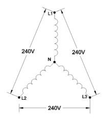
The wye transformer is occasionally wired with only three wires. In this situation, the designer has no use for the other voltage, so the center tap is unused. In this configuration, common voltages would be 240V and 480V in the US.
