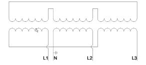
Three single phase transformers can be connected together to form a three-phase system. As a group, they raise or lower the nominal voltage of the three phase system. In this example, the primary windings are connected in a delta ( $\Delta$ ) arrangement, and the secondary wires are connected in a wye (Y). This configuration is referred to as Delta Wye ( $\Delta$ -Y). Other possible configurations are ( $\Delta$ - $\Delta$ ), (Y- $\Delta$ ), (Y-Y).
