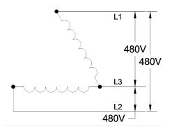
The open delta is also known as a V connection. This is a delta with one of the transformers missing. This is not a practical arrangement, but it may be used temporarily when one transformer fails. The same voltages are available, but the power is reduced by 57.7% of the original power.
