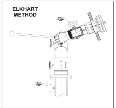
In mathematical terms, the Total Static Pressure Drop is the change in Velocity Pressure plus Friction Loss. The change in Velocity Pressure results from the change in velocity of water caused by the change in the cross section of a waterway. Friction Loss results from the drag and sidewall interference of the water through a device. A simple equation can be seen
