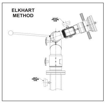
In mathematical terms, the Total Static Pressure Drop is the change in Velocity Pressure plus Friction Loss. The change in Velocity Pressure results from the change in velocity of water caused by the change in the cross section of a waterway. Friction Loss results from the drag and sidewall interference of the water through a device. A simple equation can be seen
