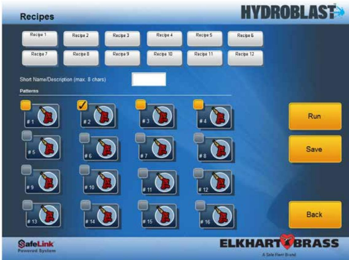
Figure 3-4 HydroBlast recipe setup screen
