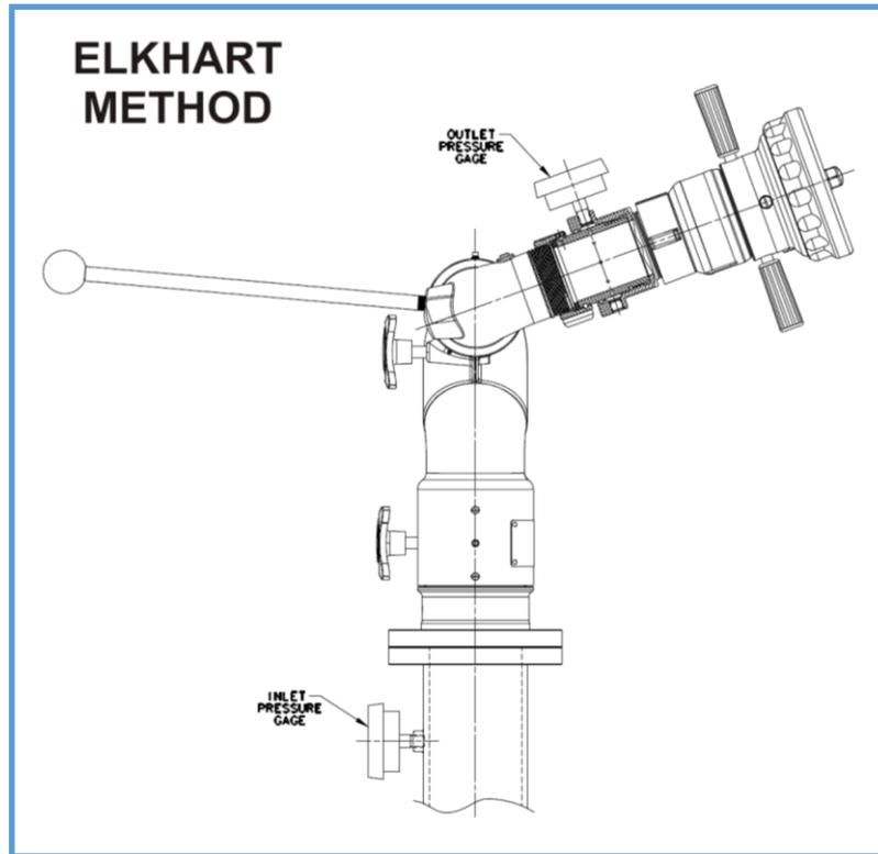
In mathematical terms, the Total Static Pressure Drop is the change in Velocity Pressure plus Friction Loss. The change in Velocity Pressure results from the change in velocity of water caused by the change in the cross section of a waterway. Friction Loss results from the drag and sidewall interference of the water through a device. A simple equation can be seen below.
