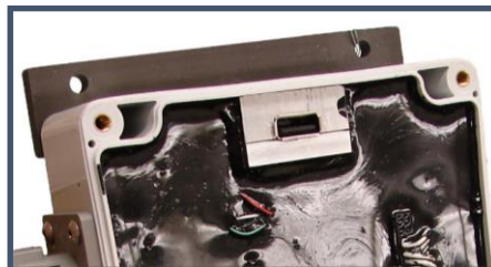
7072 OEM Interface Module - Remove the cover with a phillips screwdriver to locate the USB port.
