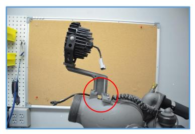
2. Remove and discard the three (3) 10-24 x 0.50" screws from the vertical motor housing.
