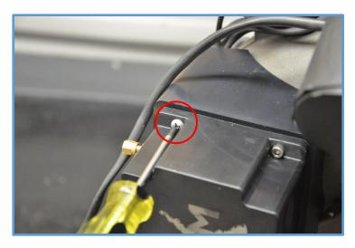
Reinstall the EXM control module to the monitor body using the three (3) previously removed 8-32 screws. Apply blue Loctite #242 or equivalent to the screw threads. Tighten these screws to 8-10 in-lbs.
