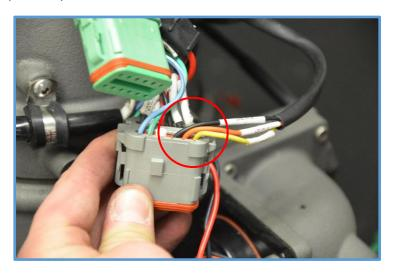
9. Reinstall the wedgelock into the 12-pin connector once all wires are securely in place.
