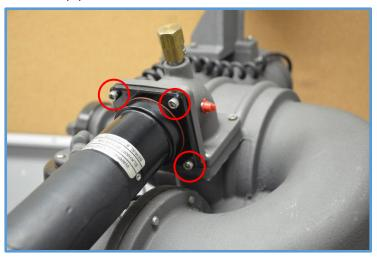
**3.** Mount the supplied light bracket to the vertical motor as shown with the supplied 10-24 x 1.25" screws. Apply blue Loctite #242 or equivalent to the screw threads.
