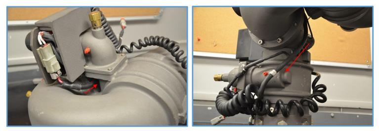
14. Remove the 10-24 screw in the location shown and clamp the light kit power harness in place with the supplied clamp loop. Apply blue Loctite #242 or equivalent to the screw threads.
