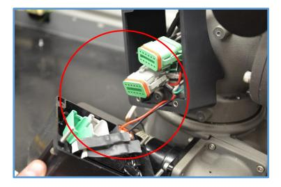
7. Remove the wedgelock from the gray 12-pin plug on the monitor harness with a small slotted screwdriver as shown. Set aside and save the wedgelock as it will be reinstalled later.
