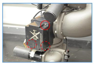
**5.** Remove the wire cover from the EXM module by removing the Phillips head screw. Save this part for later use.
