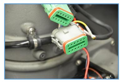
10. Route the light kit yellow, orange, and black wires along the other harnesses as shown. Slide the wire cover back over the plugs and reconnect the three (3) plugs into the EXM control module. Ensure the plugs 'click' into place.
