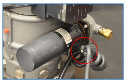
**15.** Clamp the harness from the light kit to the light bracket shown with the supplied 10-24 screw and clamp loop. Apply blue Loctite #242 or equivalent to the screw threads. Connect the light harness to the light as shown.
