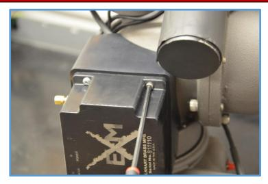
13. Route the power harness under the vertical motor and around the monitor body as shown.
