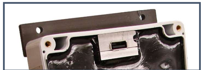
OEM Interface Module - Remove the cover with a phillips screwdriver to locate the USB port.
