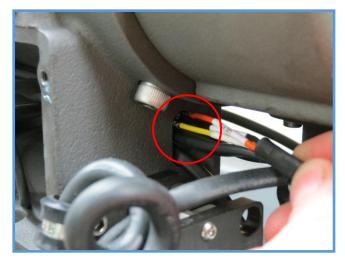
7. Remove the white cap plugs and insert the yellow, orange, and black wires into pins 7, 8, and 9 respectively. Push the wires in until a 'click' is heard, and the wires cannot be pulled out of the plug.
