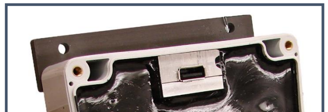
OEM Interface Module - Remove the cover with a Philips screwdriver to locate the USB port.
