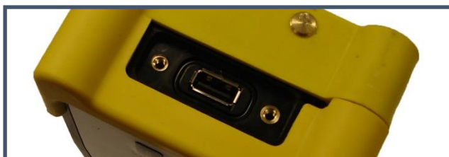
Handheld & Panel Mount - Remove the top cover on the controller with a Philips screwdriver.
