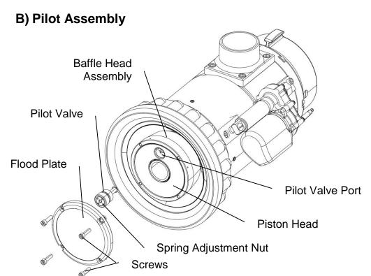
Figure 5 - Pilot Valve Assembly
