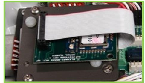
**RF Transceiver in OEM Module**
