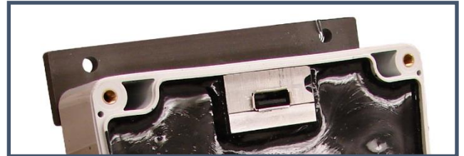
OEM Interface Module - Remove the cover with a phillips screwdriver to locate the USB port.
