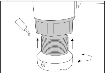
Install the quick connect inlet to base using Loctite 592 thread sealant or equivalent. Tighten using a strap wrench.
