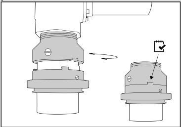
Disconnect monitor from base by pressing down on the lock ring and rotating the monitor counter-clockwise until it lifts off.
