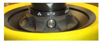
the inlet end of the nozzle will increase the flow all the way to the flush position shown in the picture while rotating the stem in the opposite direction will decrease the flow. The nozzle must be shut down before changing the flow setting.
