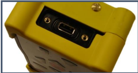
Handheld & Panel Mount - Remove the top cover on the controller with a phillips screwdriver.
