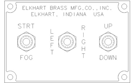
Figure 4 Primary Panel Mount Switch Module
