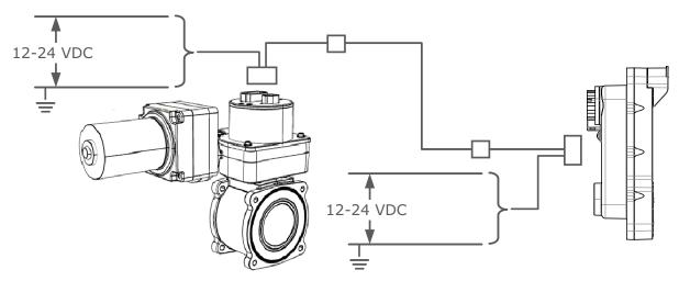
Example schematic depicting E14X or E16X actuated valve controlled via a APEX 100, APEX 200 or APEX 300 controller. See Unibody Valves general catalog pages for APEX controllers and options.
